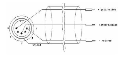
Fig. 5: Input socket for 3-pin plug
