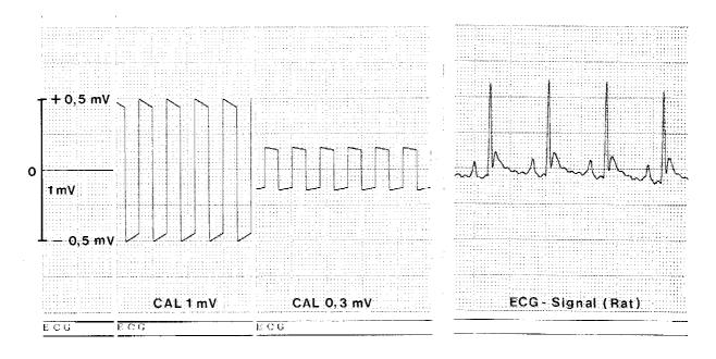
Fig. 3: Setting up an ECG scale on the chart, selected range  $\pm 1$  mV, see text above.
