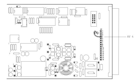
Fig. 2: Position of the internal link
